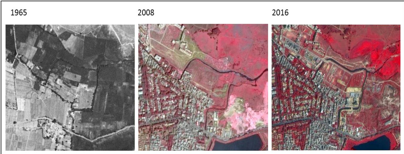
**Exhibit 3.5: Realignment of drainage network near Hosakerehalli Lake**
